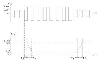
Turn on time:  $t_{on} = t_d + t_r$
